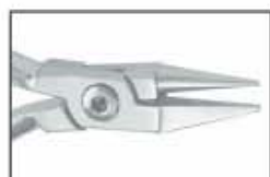
DE-1383 Bird beak plier for light wire bending round, square and rectangular up to .016"/0.41mm.
